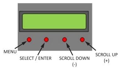
On power up the display will momentarily display "Universal Fiber Optics" then the current model version letter, then the firmware version, before going into initialisation whilst it checks the unit before displaying the current status (example below).
