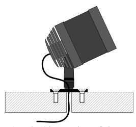
Using M5 threaded countersunk screws, fix the fitting to the mounting surface, with the cable exiting through a pre-drilled hole in the surface.
