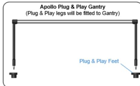
Additional central support legs are required for unsupported spans of more than 1147mm and recommended for those greater than 900mm.
