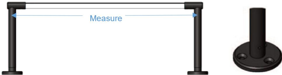
3. Use the measurement(s) to mark the centre point of each of the feet on the surface where the Gantry will be mounted. If there are more than two legs, ensure marks are in a straight line to avoid straining the Apollo's structural components.
