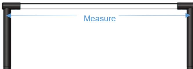
3. Use the measurements to mark the centre point of each of the feet on the surface where the Plug & Play Gantry will be mounted. If there are more than two legs, ensure marks are in a straight line to avoid straining the Apollo's structural components.
