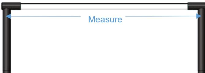
3. Use the measurement(s) to mark the centre point of each of the feet on the surface where the Gantry will be mounted. If there are more than two legs, ensure marks are in a straight line to avoid straining the Apollo's structural components.
