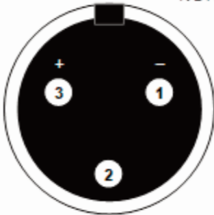
Male – for connection to lower (female) Gemini Mini-XLR socket
